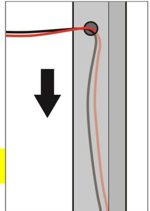
8. Make sure the wires can reach the power source. Trim off any excess length if needed. Attach the Male Spade Connector to the red wire (+12V or 48V) coming out of the fan. Attach the Ring Terminal to the black wire (-12 or 48V).
