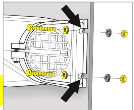
**CAUTION:** Do not overtighten hardware as it can cause damage to the floor and/or the RHOXAir mounting brackets.
