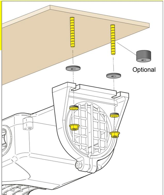
6. Use an oscillating or reciprocating saw to trim off any excess bolt length from the (4) mounting bolts. Leave at least a 1/4" of exposed threads on the bolt.
