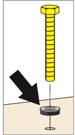
5. Place the (4) Rubber Washers between the top and the fan as shown. Install the RHOXAir fan to the top using (4) 6mm Serrated Flanged Locknuts and (4) 6mm Metal Bonded Sealing Washers. Use the 6mm x 13mm Thick Rubber Spacers to provide more angle if needed. Hand tighten hardware.
